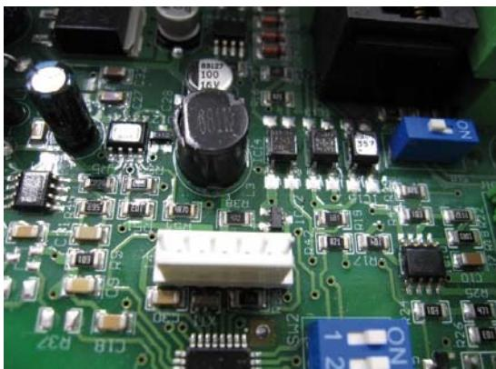
4. Line up electronic component TIMER RTC ECOWATT with J4 connector pins
