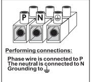
All the Heated Air Curtains with electric heating work with a three-phase alternating-current mains 400 (+10 %) V, 50 Hz with Neutral and Grounding. The cable is connected to the terminals located inside the unit.
