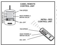
All Recessed OLEFINI Air Curtains have a wired-infrared remote control, allowing to switch ON-OFF the device, to change fan speed, to change heating efficiency (HEAT POWER) or to control the hot water solenoid valve (WATER VALVE) depending on the way of heating.
