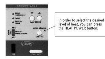
By pressing this button once you step to the next level of heat. Once 100% heater power has been achieved, one more press will switch to Non Heaters mode
