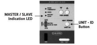
To change the ID of a unit, it is necessary to first TURN OFF the unit and wait until it is completely off (the fan is turned off and depending on the current ID, the MASTER/SLAVE LED is on or off. All other LEDs are off).
