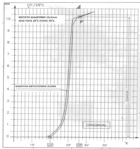
ly less than 20°C in cooling and more than 28°C in heating we can use this phenomenon with a proper motion transmission mechanism to adjust automatically the blades corner in the values calculated by the diagrams of the previous pages.
