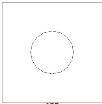
When we want to install the diffusers MLD, MLD-DW in false ceiling with dimensions 600X600 mm we can use the plate SPR.
