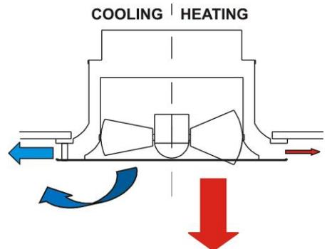
In the MLD type swirl diffuser while the blades are being closed the pressure drop and the noise increase, because the free surface of the diffuser decreases. So, the pressure drop and the noise in cooling are higher than heating. This takes place too little in the MLD-DW type, because of its double wall design, while at the same time the vertical throw in heating is not affected (so long as the blades are in a little more vertical position than the blades of simple MLD).
